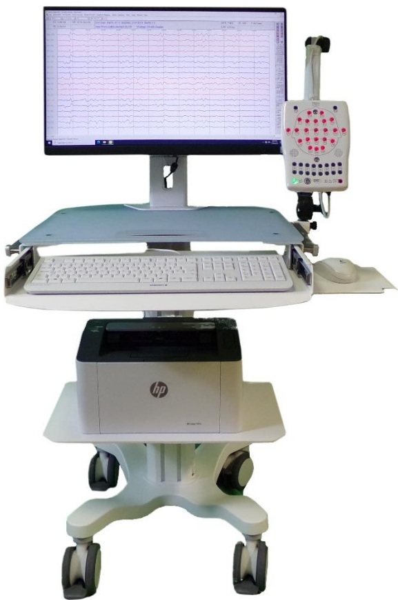
Trolley (height adjustable) based routine EEG workstation (with 10/20 LED headbox)
